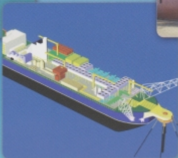
5,000 Ton Per Day Gas to Methanol FPSO: Designed and model-tested the world's largest proposed floating methanol plant ship for the US DOT.
