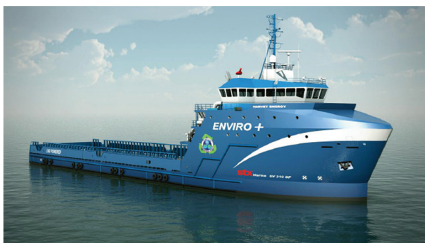
Figure 2. Harvey Gulf's LNG-fuelled US flag offshore supply vessel.
